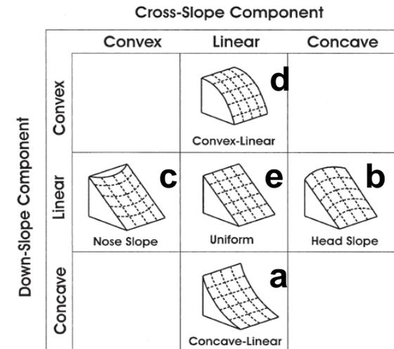
Fig. 1. Cross-slope and down-slope components of the flume experiments including naming convention. At the flume outlet all shapes were linear due to the design of the experimental box. Only components with at least one linear component could be used.
