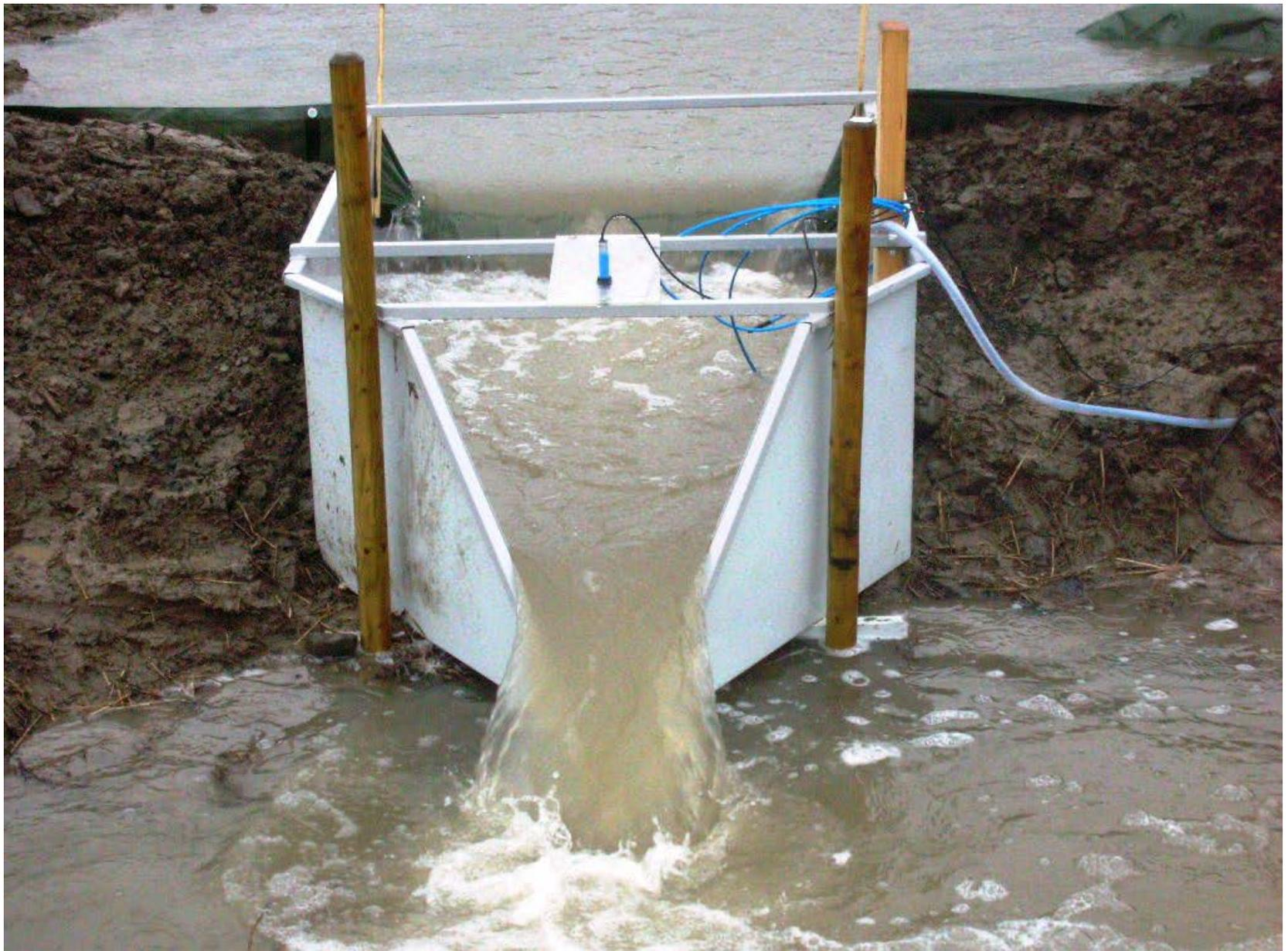
H-flume with a "Ultrasonic flowmeter", at a field in Skaterud catchment, Norway
