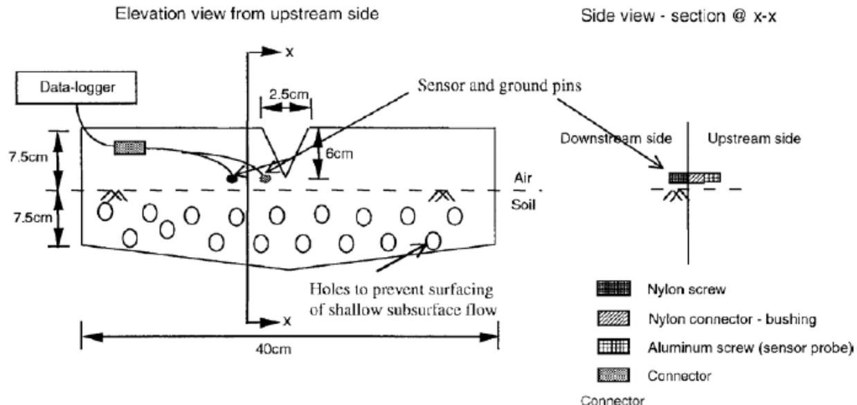
A water bridge between the sensor and ground pins triggers the circuit and gives a signal of 1.8 V.
